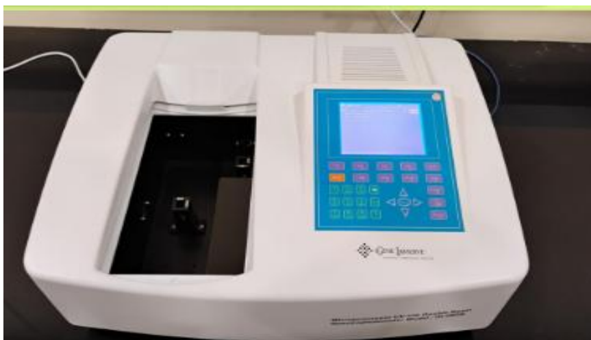
Figure 1: Microprocessor UV-VIS Double Beam Spectrophotometer (IG-28DS)
